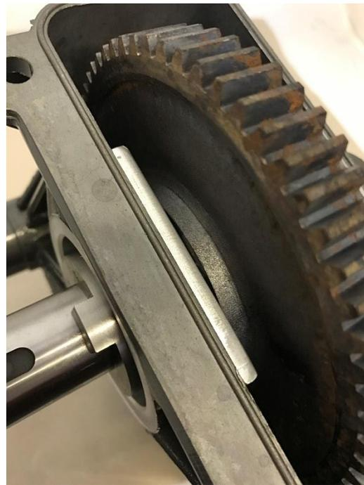
Be certain that the circlip is correctly fastened and that the bronze bush and oil seal are correctly re-fitted, and re-fit the brake assembly to the mainshaft. If the winch had the three spring disc washers behind the circlip, then re-fit these, and then fit the mainshaft end cap with the M12 schnorr washer and Cap Head bolt. Ensure that the bolt is tight.
