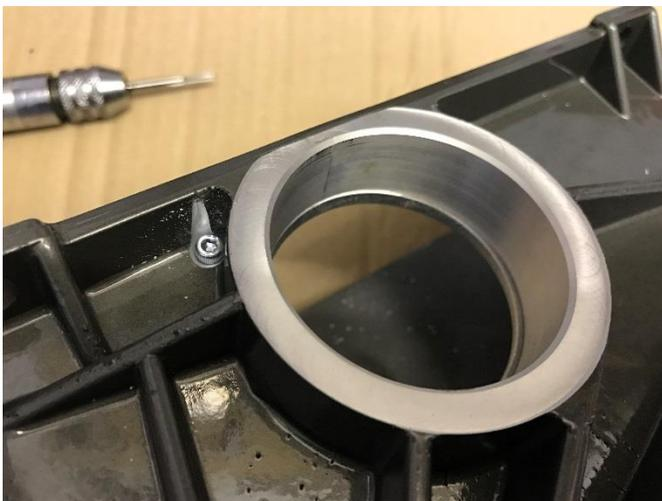
Before fitting the shim to the casing, use a 3.5mm drill bit to widen the holes in the casing.
