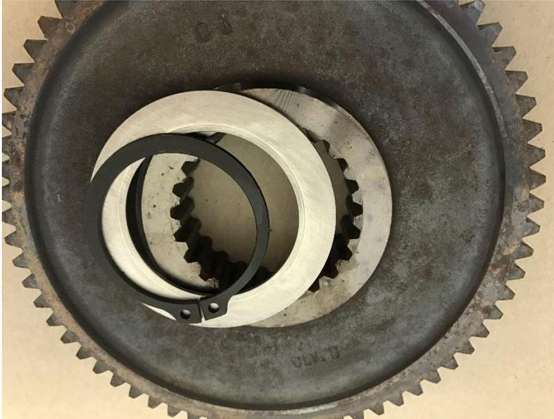
Now slide the two cam gears over the mainshaft (fitting the O Ring first) and insert the mainshaft, taking care to fit the large intermediate gear, round shim and circlip.
