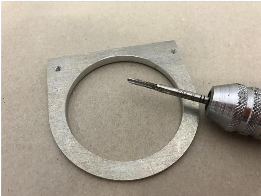
Remove the shim from the casing and using the supplied M3 tap, tap the 2 holes in the shim (WD40 can be used as a lubricant).
