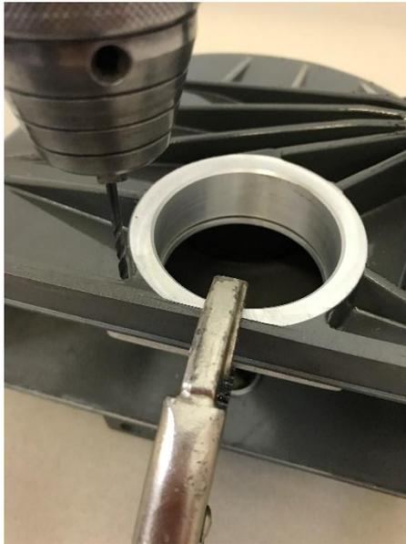
After carefully checking the alignment, use the existing holes as a guide to drill through the casing and shim together using a 2.5mm drill bit.
